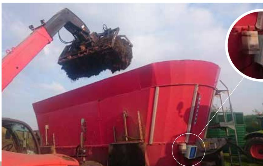
NIR analyzer for feed mixers' tank
