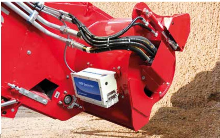
NIR analyzer for self-propelled feed mixer
